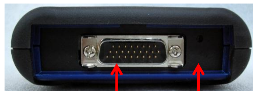
1. OBD cable connector 7. Diagnosis led status
